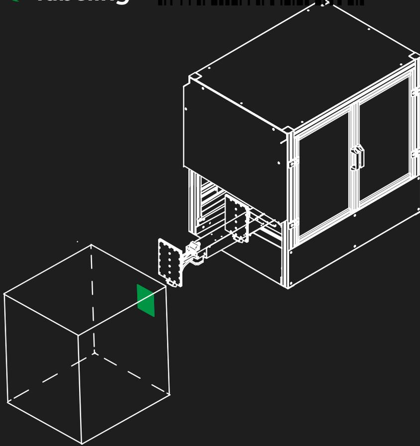
AP182 is an automatic print & apply system, suitable for A5 labels application on multiple sides of a pallet, according to the international logistic identification standards. The complete system is enclosed into a robust aluminium frame to be protected from dust and dirty environments.
